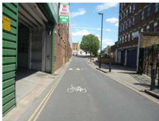
Diagram 1057 symbols showing continuation of cycle route and recommended road position
