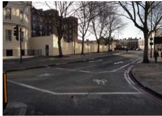
Use of a, irregularly shaped ASL reservoir where an island separates movements
