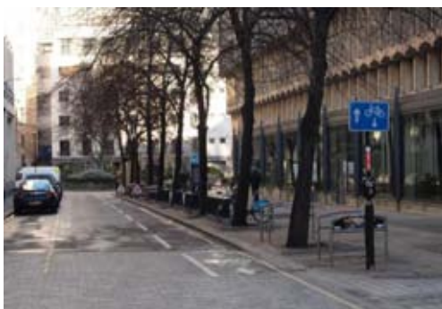
Contraflow cycling in City of London using the diagram 960.2 sign: advisory contraflow at Aldermanbury Street (left) and at Noble Street (right) using advisory lane markings only at the junction
