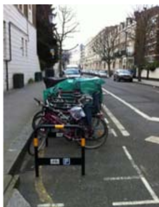
Cycle stands should not create new hazards for pedestrians: use of on-carriageway space for cycle parking
