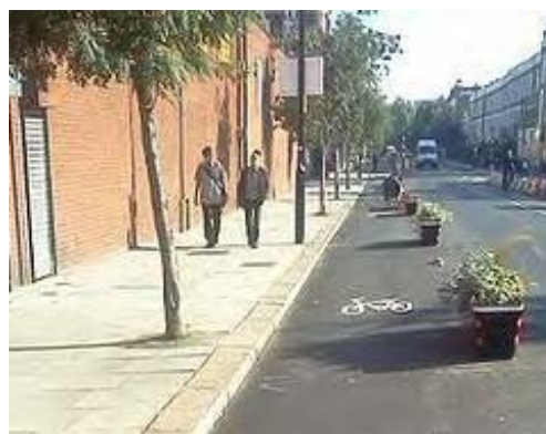
(Left) cycle tracks that break to become lanes across accesses and side roads and (right) space for cycling delineated by objects – technically, neither a lane nor a track
