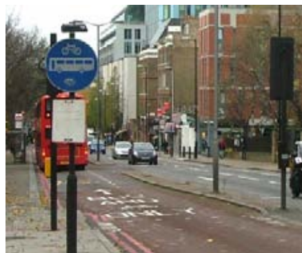
With-flow bus lane (left) and contraflow lane with 'bus and cycle' marking (right)
