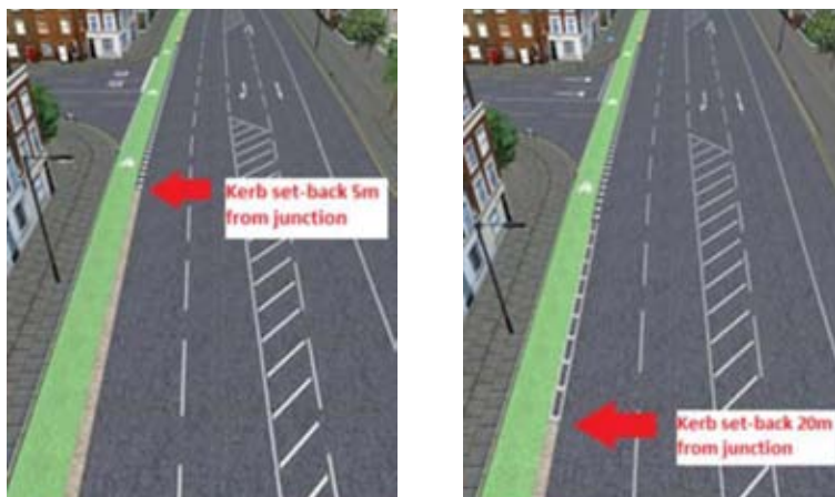
Diagrams showing segregation setback distances trialled off-street
