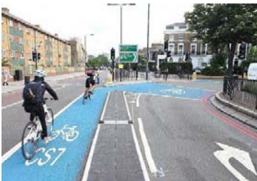
Offside protection on central lead-in (left). Offside lead-in lane (right)
