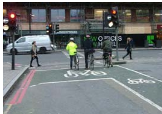
Offside protection on central lead-in (left). Offside lead-in lane (right)
