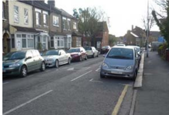
Gaps force cyclists to deviate from their line and into the door-opening space of parked cars
