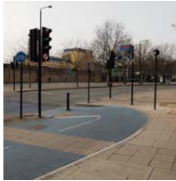
Type [1]: parallel crossings at Westferry and West India Dock Road. Ladder and tramline tactile paving are used for transition from track to shared area.
