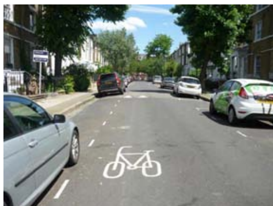
Diagram 1057 symbols showing continuation of cycle route and recommended road position
