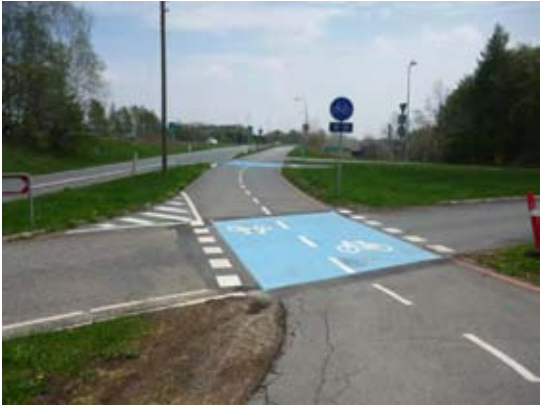
Elephants' footprints markings and surface colour used to highlight conflict point as cycle route crosses the carriageway (Copenhagen)
