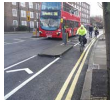
Cycle lane with buffer and intermittent island protection – Baylis Road, Lambeth
