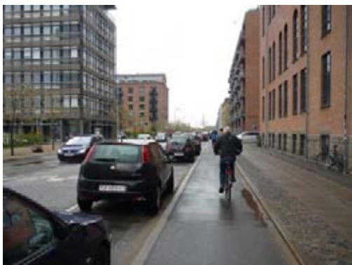
Stepped cycle track in Copenhagen – small, clear level difference between footway and cycleway
