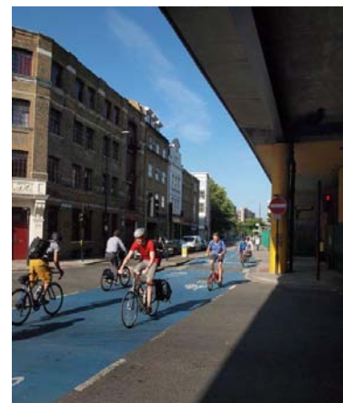
At least 3m width needed for comfortable two-way cycling Cable Street, Tower Hamlets
