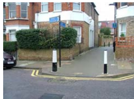
There is insufficient width to allocate sides of this cut-through to different users, so shared use makes more sense
