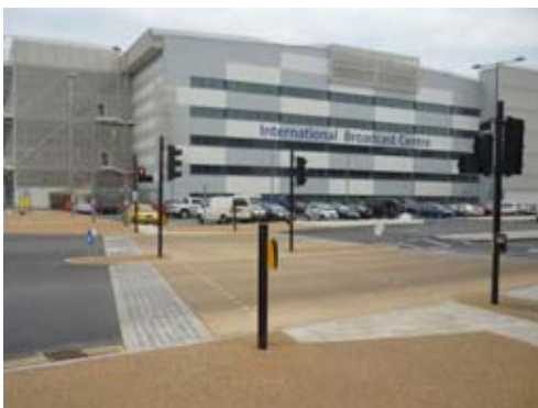
Crossing on a raised table and with contrasting surface treatment, Waterden Road, Hackney
