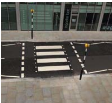
Conventional zebra crossing (left), with buff blister tactiles. Shared area on either side of the zebra (right) to legitimise cycle use of the crossing.
