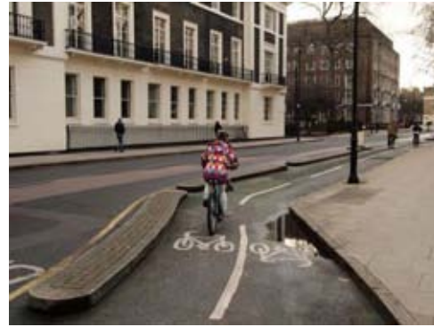
Two-way facilities can lead to awkward transitions when joining with one-way provision (left) Consideration needs to be avoiding pinch-points at bends where effective width is squeezed (right)
