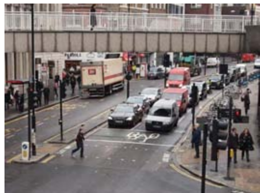
Traffic lanes narrowed to incorporate nearside feeder to an ASL – Aldersgate Street, City of London
